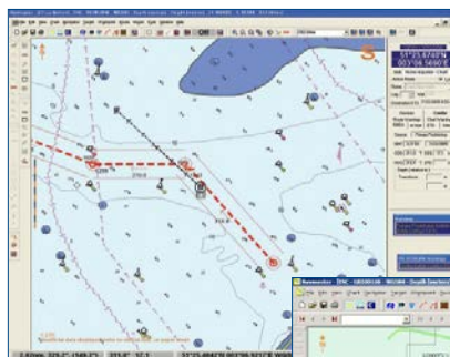
VESSEL UNDERWAY WITH HEADING MARKER SHOWING PREDICTED POSITION AT USER-DEFINED INTERVALS.
